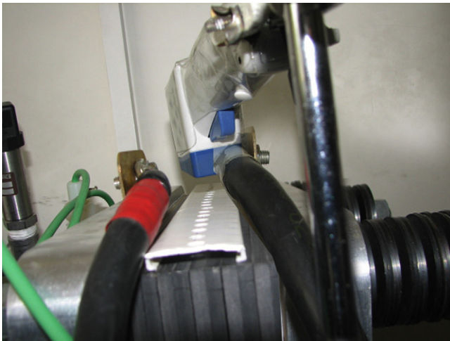
Fig. 2. Temperature measurement of the bipolar plate edges by the infrared thermometer.
